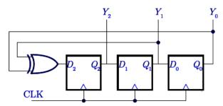
4. The outputs of the two flip flops Q1 and Q2 in the figure shown are initialized to 0, 0. Find the sequence generated at Q1 upon the application of clock signal.
